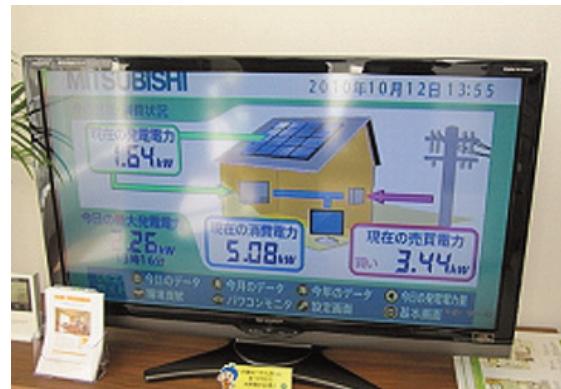
PV metering & grid interaction/sales monitoring system hooked up to the television
